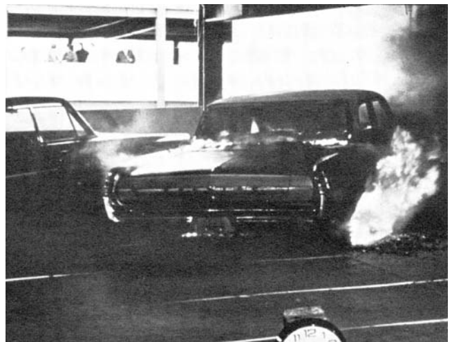
Fig. 8.1. Burning Automobile After 24 Minutes in 1972 Scranton Fire Test of Parking Garage (Gewain, 1973) (Modern Steel Construction, 1973)
